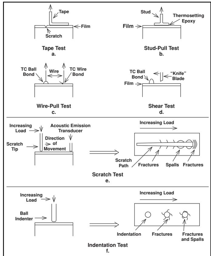
Figure 1: Adhesion tests. a) Tape test; b) Stud-pull test; c) Wire-bond and ball-bond pull test; d) Shear or topple test; e) Scratch test and scratch pattern; and f) Indentation test and indentation patterns.
